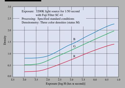
In order to simulate conditions closest to practical use, exposure was made under a 3200K tungsten light source, through a Fuji SC-41 ultraviolet absorbing filter. Processing was carried out under standard conditions and the three color densities were measured, producing the results indicated here.
