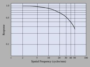
\* Spatial frequency attenuation characteristic of amplitude relative to rectangular wave chart.
