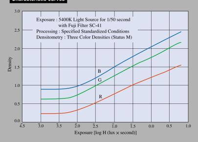
In order to simulate conditions closest to practical use, exposure was made under a 5400K light source, through a Fuji SC-41 ultraviolet absorbing filter. Processing was carried out under standard conditions and the three color densities (status M) were measured. The results of measurements are plotted as characteristic curves.
