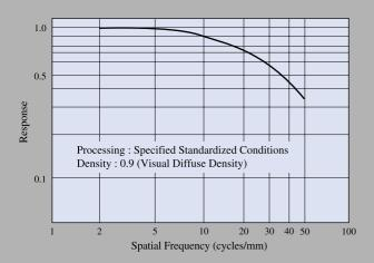
\* Spatial frequency attenuation characteristic of amplitude relative to rectangular wave chart.
