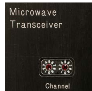
Channel Selector Switches
