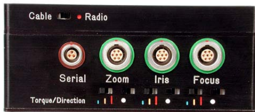
MDR2: Torque and Direction Switches
