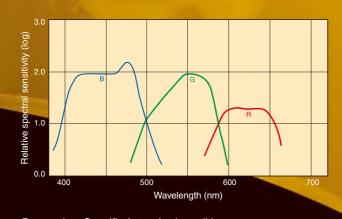
Processing: Specified standard conditions Densitometry: Arbitrary three color densities Density: 0.40 above minimum density Sensitivity: Reciprocal of exposure (ergs/cm<sup>2</sup>) required to produce specified density
