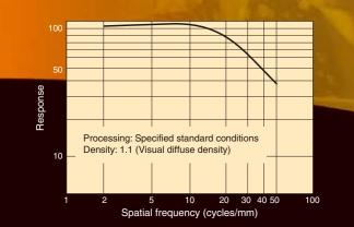
\* Spatial frequency attenuation characteristic of amplitude relative to rectangular wave chart. (Data is normalized for amplitude of zero frequency.)
