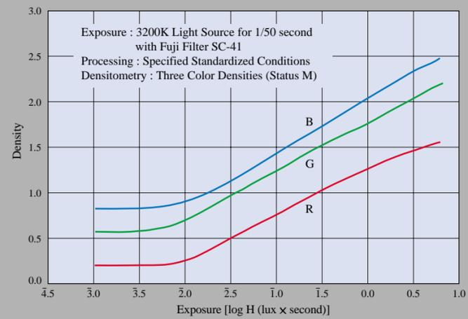
In order to simulate conditions closest to practical use, exposure was made under a 3200K light source, through a Fuji SC-41 ultraviolet absorbing filter. Processing was carried out under standard conditions and the three color densities (status M) were measured. The results of measurements are plotted as characteristic curves.
