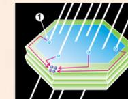
Diagram of thin-hexagonal silver halide grain
