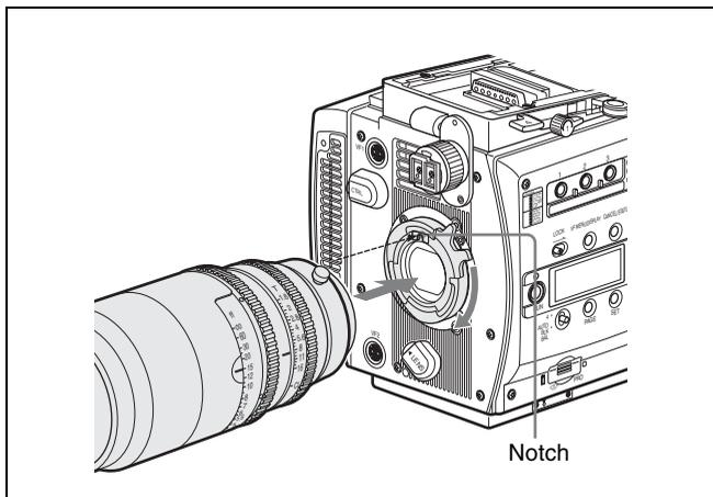
When a lens with a lens cable has been mounted, connect the cable to the LENS connector located at the lower left of the lens mount.
