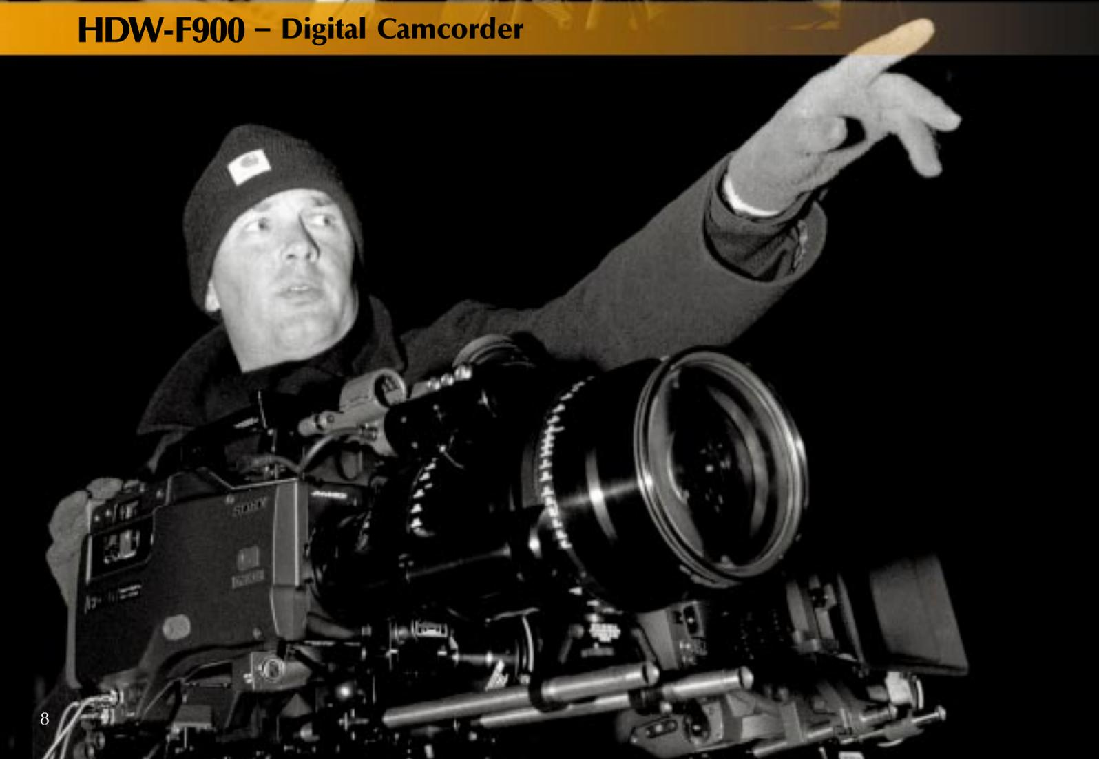
The HDW-F900 digital HDCAM camcorder combines a 3-CCD HD color digital camera, where each RGB imager has 1920 (H) x 1080 (V) sensors, with an HDCAM compact digital 1/2-inch cassette recorder. These superb new CCDs, a 12-bit A/D converter and advanced DSP processing combine to make a camcorder ideal for digital cinematography. The introduction of new techniques of HD signal processing improves the image quality even further while also simplifying the overall setup operation.
