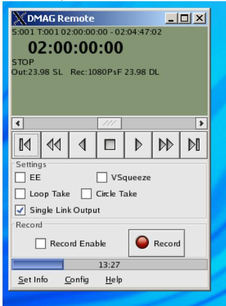
The upper line on the main timecode screen shows the scene number followed by take number followed by start and stop timecode of the current scene. The large numbers show current timecode location and increments in play and record.
