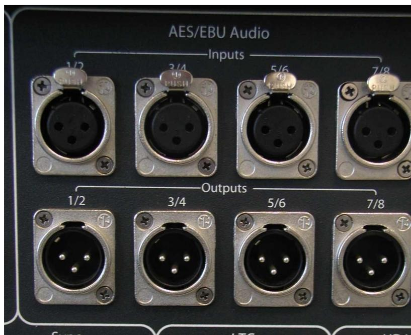
**Figure 15 Audio I/O section**
