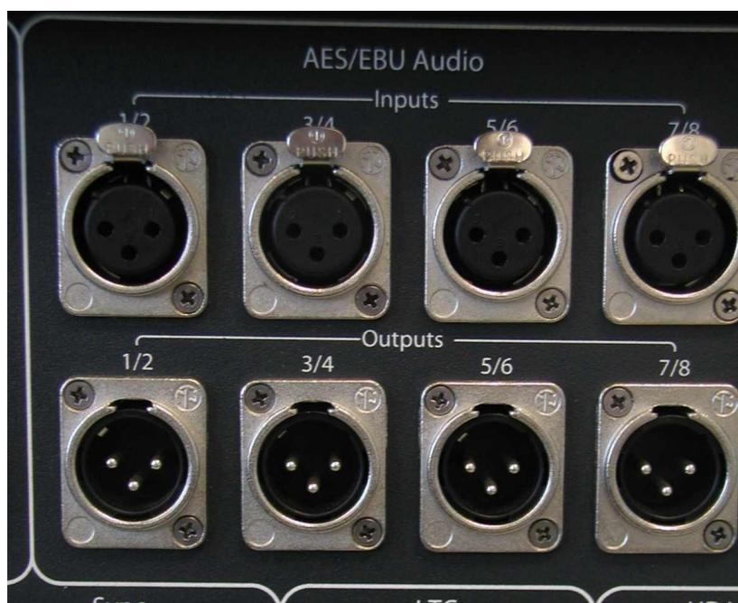
**Figure 15 Audio I/O section**
