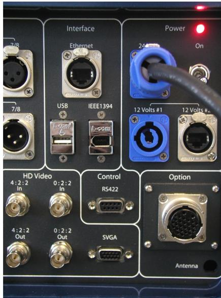
Power connections on the DFR are 24V DC. The voltage is internally regulated and will accept a range of 22V DC to 36V DC. The DFR has two Neutrik 'PowerCon' connector for 24V. This allows for battery change over when in the field avoiding power cycles in a long record.
