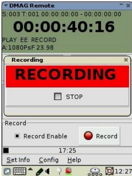
The RECORD button is not armed unless the user has enabled record. This is set using the RECORD ENABLE button. If record is armed a touch of the RECORD button will initiate a record sequence and start the record the timecode will roll.
