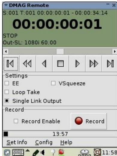
1. Power ON the iPAQ PDA. Touch the screen to activate the primary display. Use the lower left button to access the DMAG Remote program
