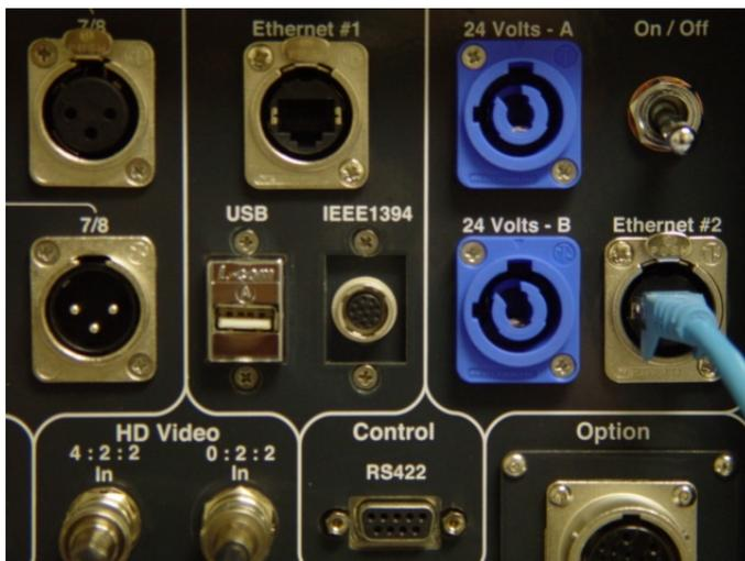
DFR Connection panel showing optional LCP remote connector that replaces the IEEE1394
