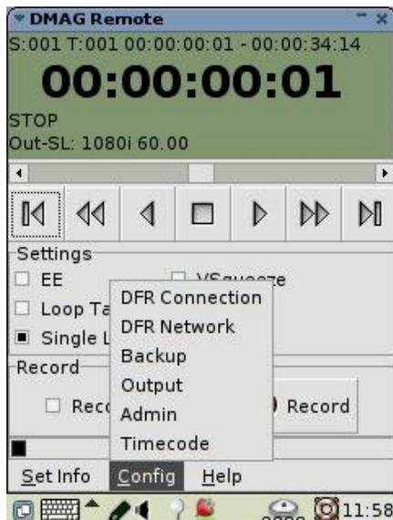
The Config Menu leads to various configuration set up menus, DFR Connection, DFR Network, Backup, Output, Admin and Timecode.
