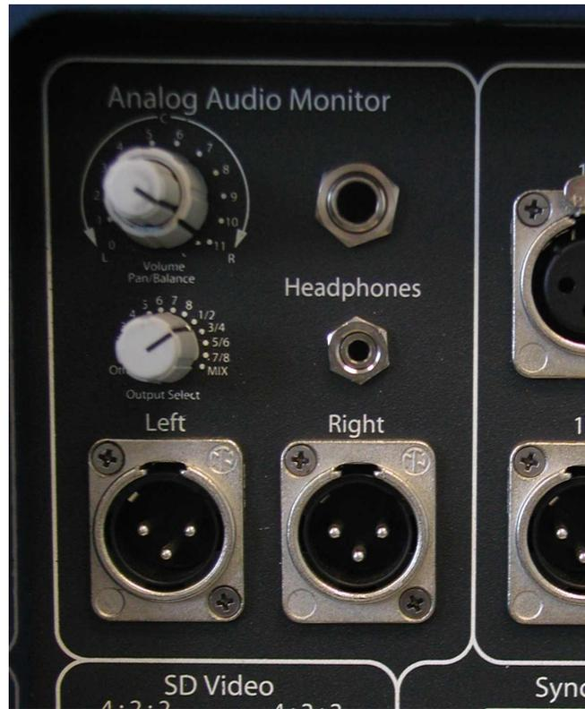
**Figure 16 Audio monitor section**
