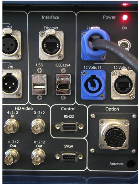
**Figure 10 Power connections**
