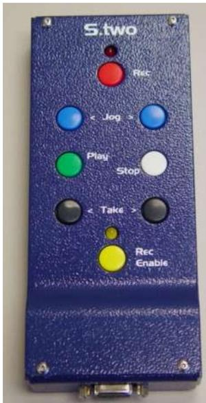
Using the LCP assumes that the DFR is already set up for frame rate, image size, outputs, color space and timecode. These can be set with either the PDA or laptop as normal.
