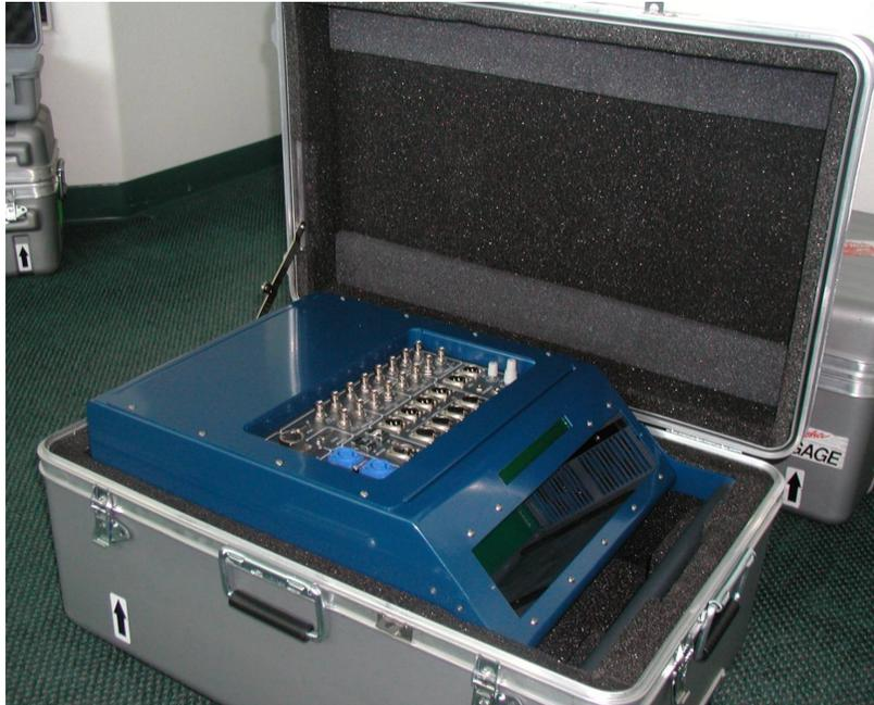
The DFR is designed to be a robust, portable unit and has been tested for common carrier shipping (Fed-EX, UPS, DHL etc.) throughout the World.
